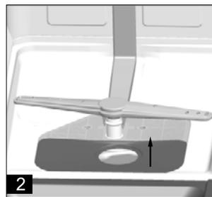
NOTE: If operate from step 1 to step 2, the filter system will be removed; while operate from step 2 to step 1, the filter system will be installed **3**.
