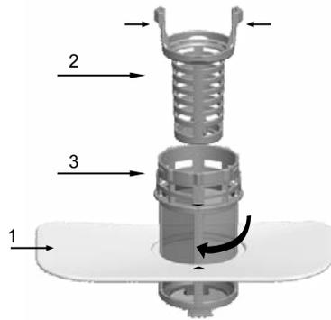
The filter system consists of a coarse filter, a flat (Main filter) and a micro filter (fine filter).
