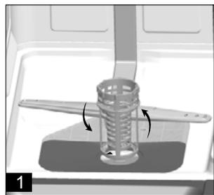
Step 1: contrarotate the Coarse filter, and then lift it up;
